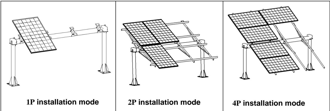
Risen module can be installed and used on the tracking system, and the installation hole position or clamp position shall be selected according to the design of the support system. Please refer to section 8.1 ,8.2 and 8.3 for details;
